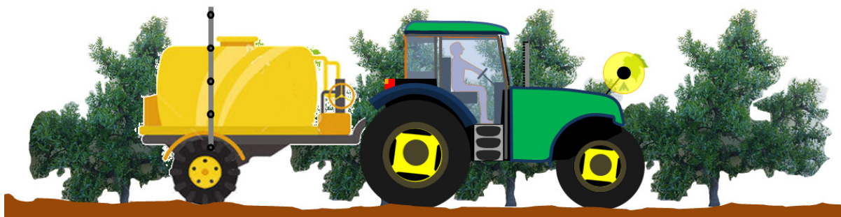
Fig. 1. Schematic representation of a three-dimensional sensor unit, positioned in front of the tractor for a feed-back system, allowing variable rate distribution with the implement
